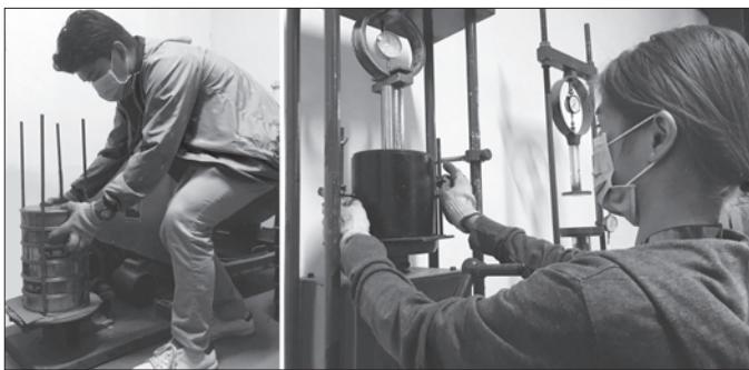
UC Civil Engineering students utilize the sieves (left) and the California Bearing Ratio molds and apparatus (right). These equipment are acquisitions of the UC College of Engineering and Architecture Materials Testing Laboratory which allows students to apply practical Civil Engineering practices in the conduct of their experiments and researches.
